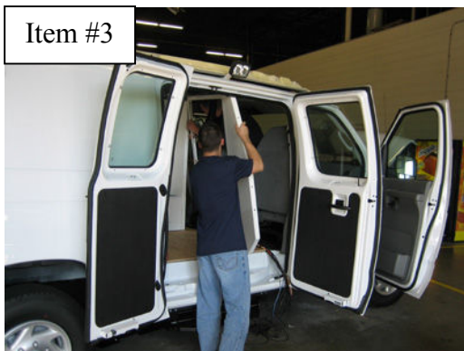
Place Front Bulkhead into vehicle
